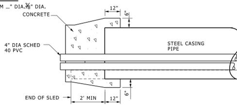
**METHOD FOR SEALING CASING ENDS**
