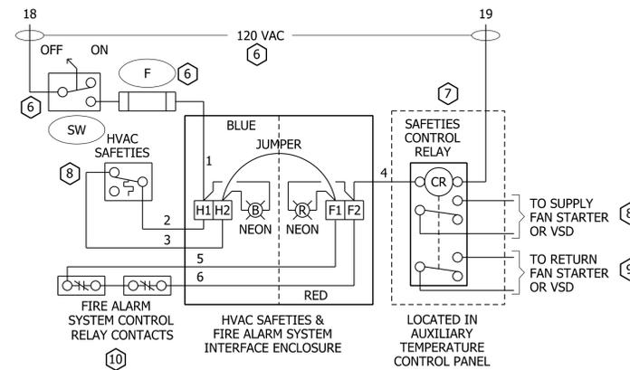
**INTERFACE BOX WIRING DETAIL**
