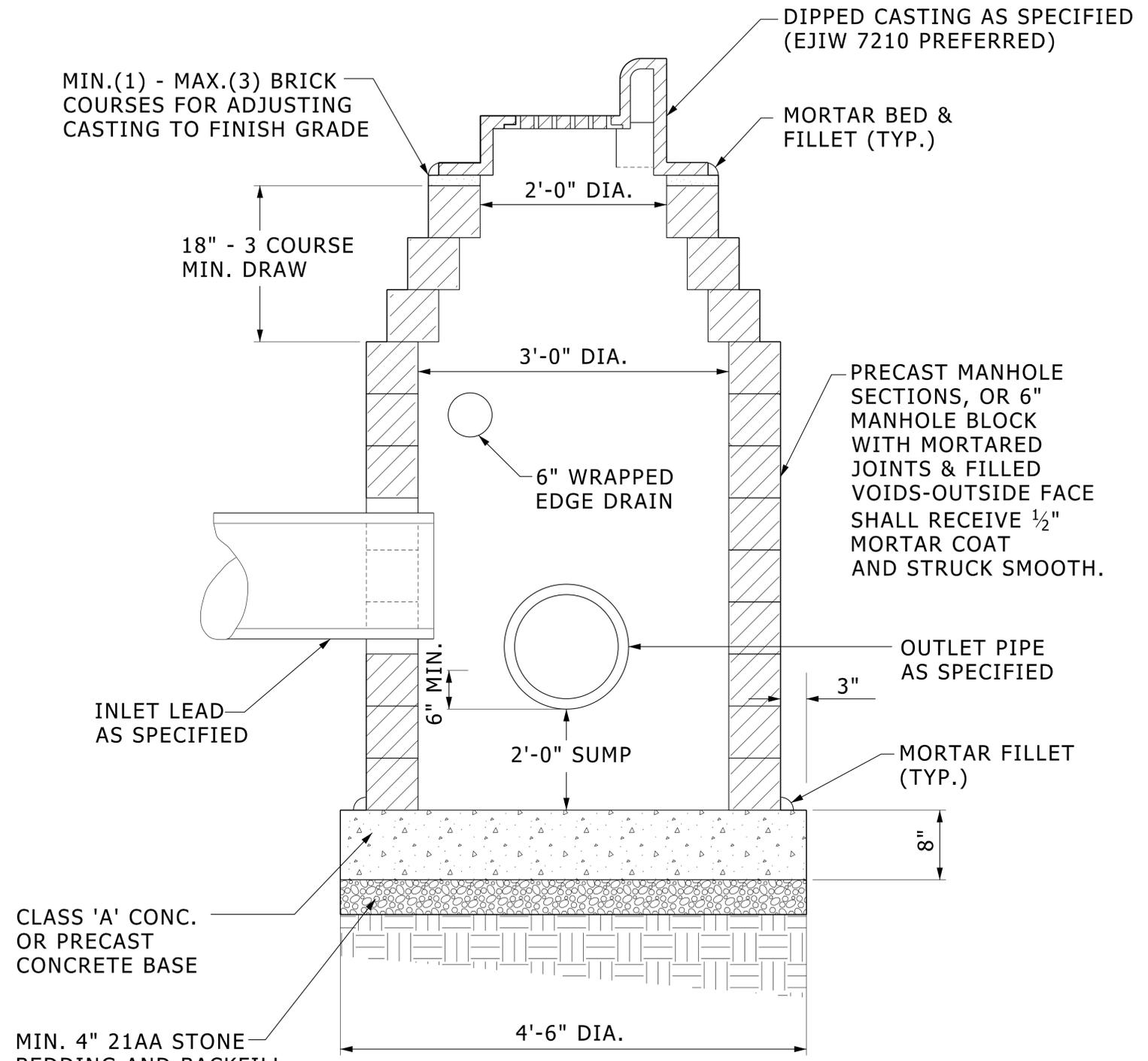
NOTE: THIS STRUCTURE SHALL BE USED IF SINGLE OUTLET PIPE AND SINGLE INLET PIPE
