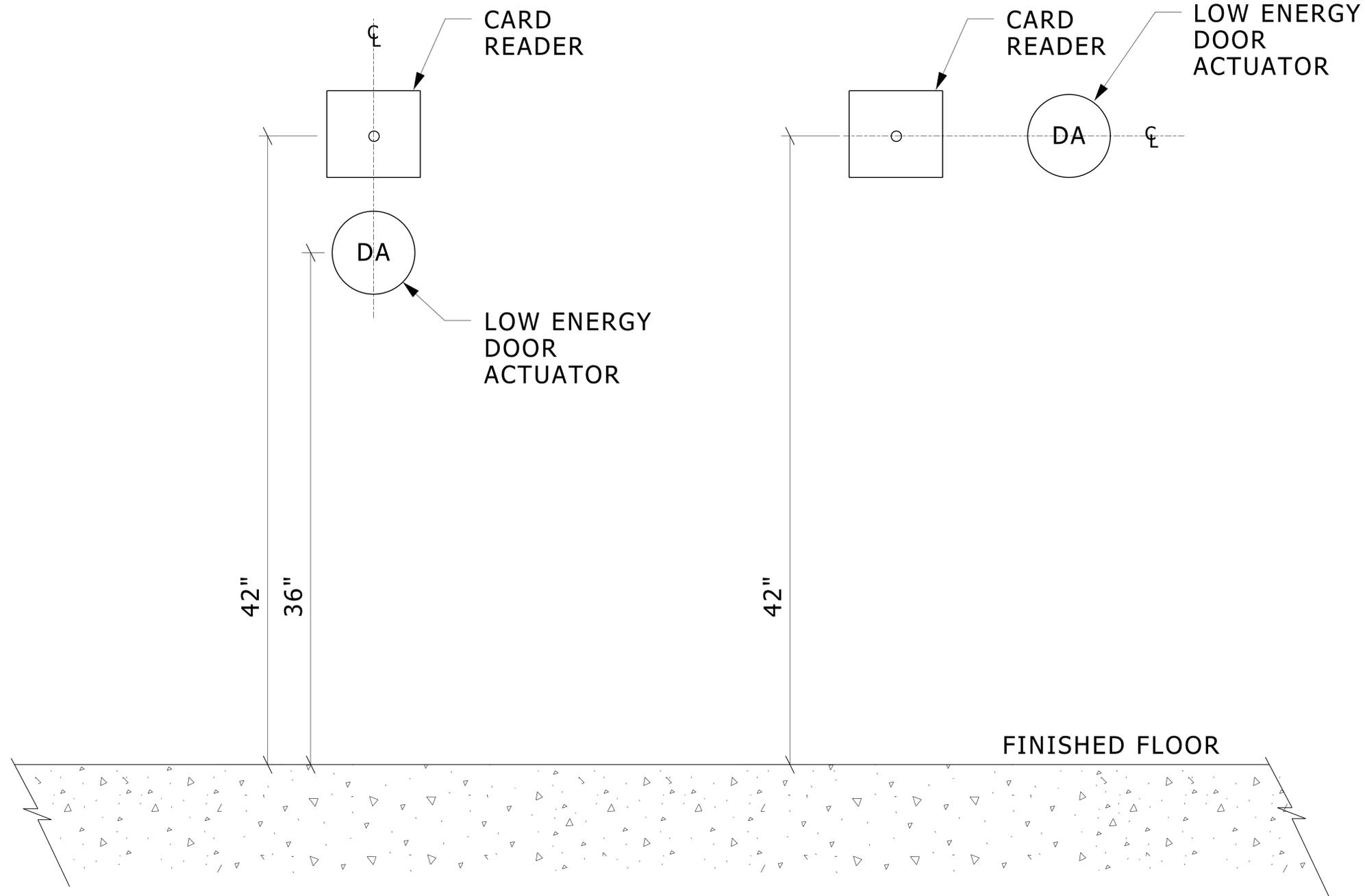
**TYPICAL CARD READER AND DOOR ACTUATOR MOUNTING DETAIL**
