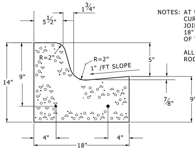
NOTES: AT 90° ANGLE POINTS IN THE CURB LINE, PLACE EXPANSION JOINTS IN THE "LONG LEG" - 18" FROM THE BACK-OF-CURB OF THE "SHORT LEG."
