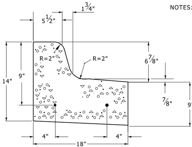
NOTES: AT 90° ANGLE POINTS IN THE CURB LINE, PLACE EXPANSION JOINTS IN THE "LONG LEG" - 18" FROM THE BACK-OF-CURB OF THE "SHORT LEG."
