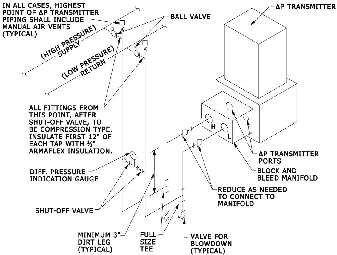
IN ALL CASES, HIGHEST POINT OF ΔP TRANSMITTER PIPING SHALL INCLUDE MANUAL AIR VENTS (TYPICAL)
