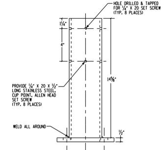
**DETAIL C - LIGHT FIXTURE BASE FIVE GLOBE FIXTURE**
