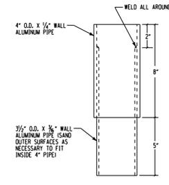
**DETAIL B - LIGHT FIXTURE BASE EXTENSION SINGLE GLOBE FIXTURE**
