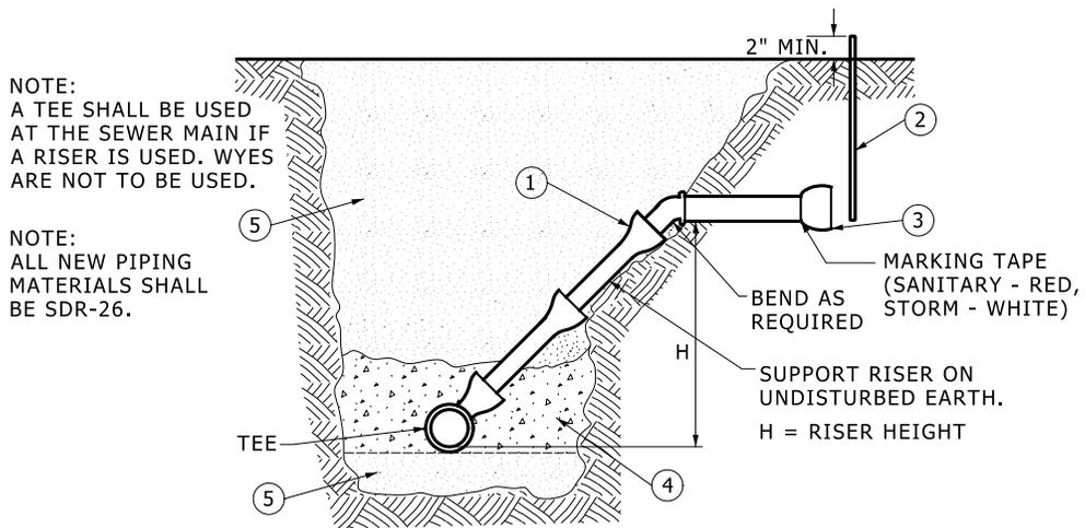
1. CARRY TO WITHIN 8' TO 10' OF GROUND ELEVATION.
