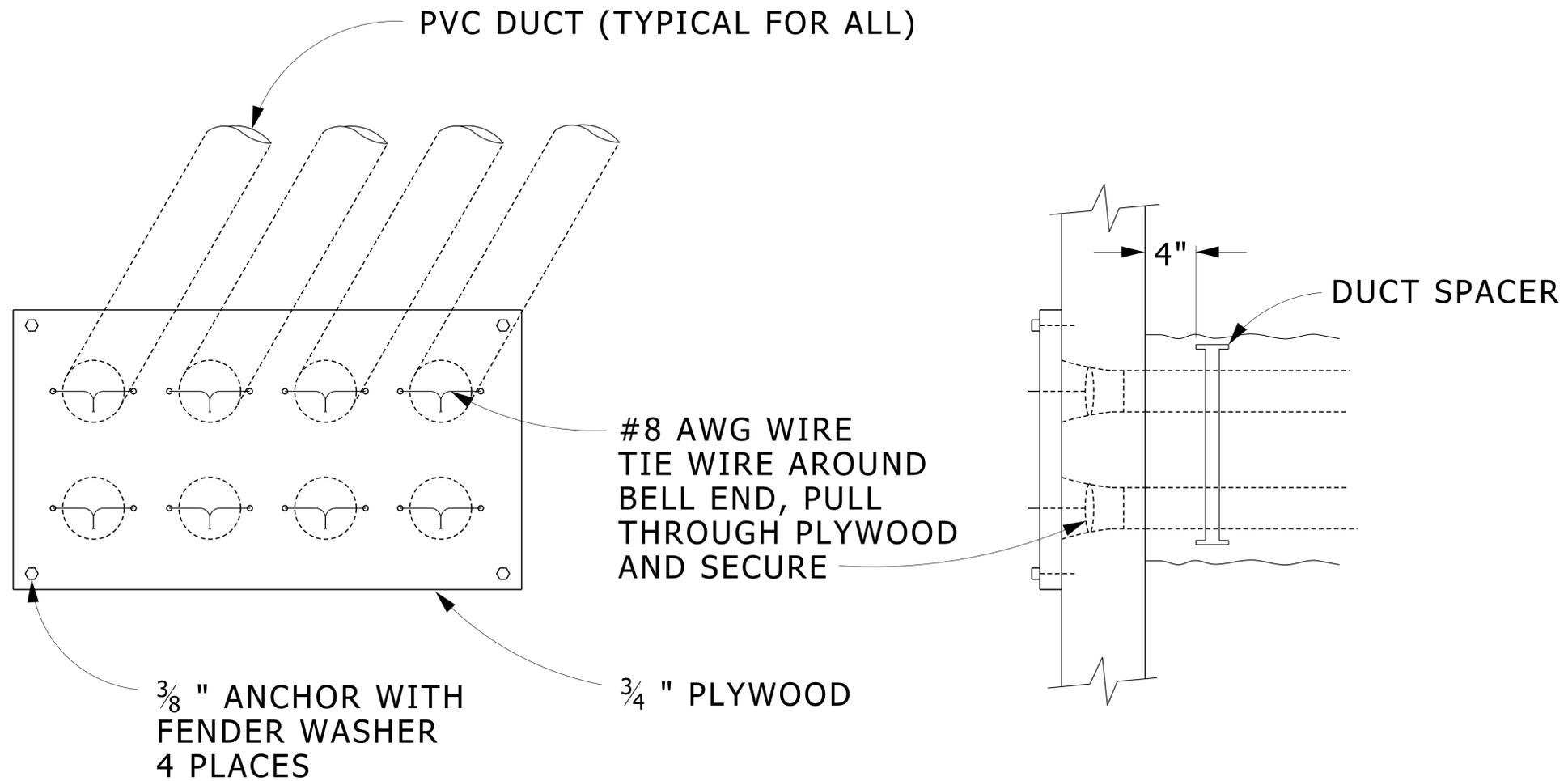
1. DUCT RUNS SHALL EXIT AND ENTER MANHOLES IN SAME SYMMETRICAL CONFIGURATION. DUCTS SHALL CORRESPOND AS MIRROR IMAGE FROM ONE END TO THE OTHER.
