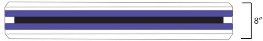
1-1/2" x 1-1/2" stainless steel square tube frame on which the panels are hung
