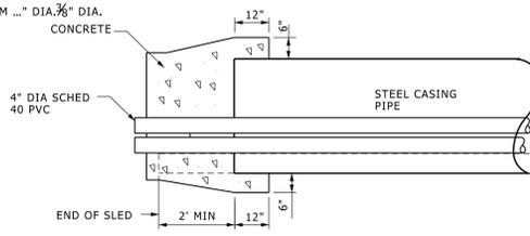
**METHOD FOR SEALING CASING ENDS**
