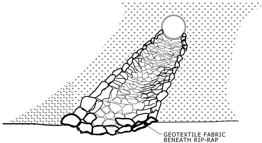
1. MATERIAL USED FOR RIP- RAP SHALL BE SOUND, TOUGH, DURABLE AND FREE FROM STRUCTURAL DEFECTS, AND MAY CONSIST OF STONE, ROCK, COBBLESTONE OR BROKEN CONCRETE WITH AT LEAST ONE DIMENSION OF 8 INCHES AND A VOLUME OF NOT LESS THAN  $\frac{1}{3}$  OF A CUBIC FOOT. SMALLER PIECES MAY BE USED FOR FILLING VOIDS AFTER LARGER PIECES HAVE BEEN SET.
