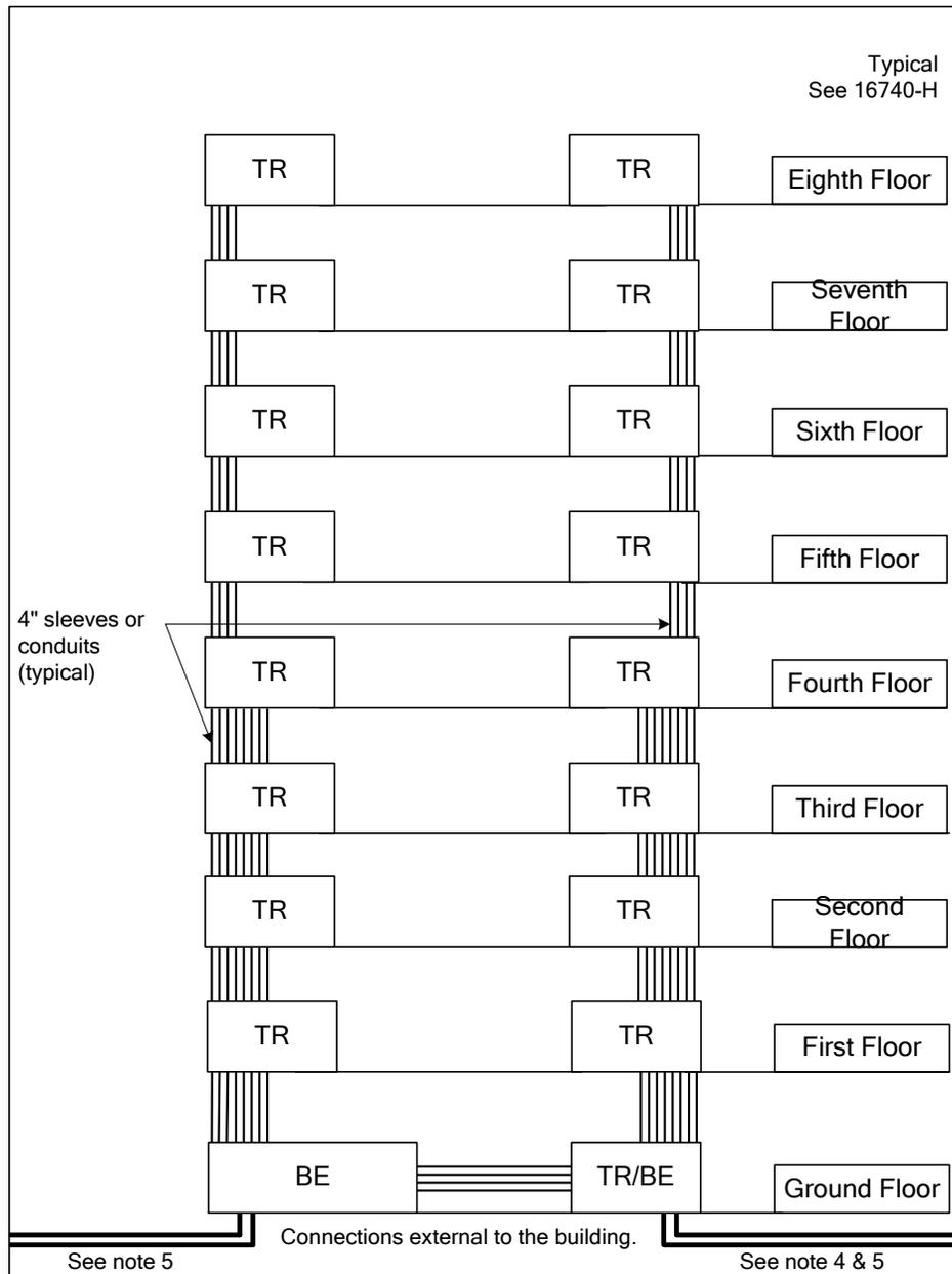
**Figure 1 – Typical Building BE/TR Room Riser Diagram**
