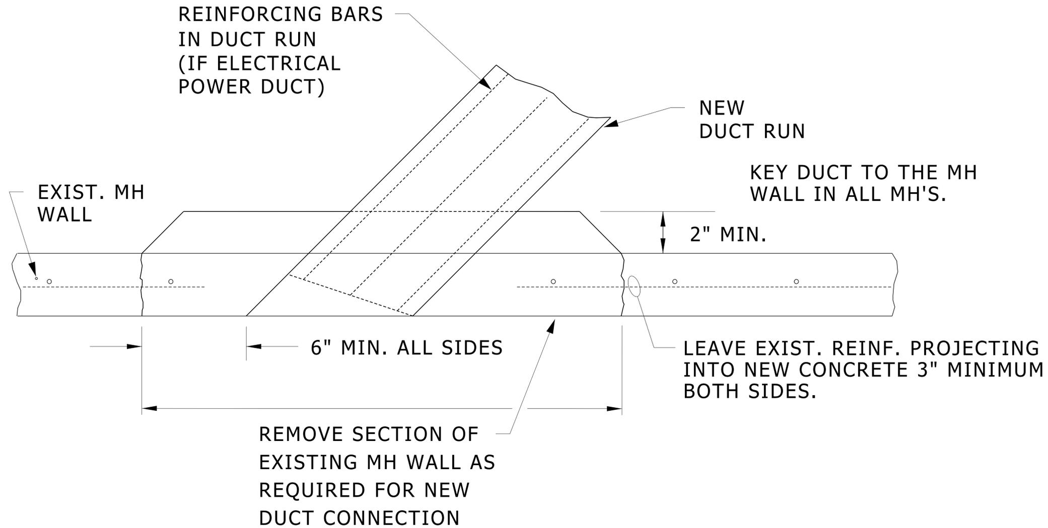
NOTE: ENTRANCE INTO NEW MANHOLE TO BE SIMILAR. LEAVE OPENING IN NEW WALL WITH REINFORCING PROJECTING, TO RECEIVE NEW DUCT CONSTRUCTION.
