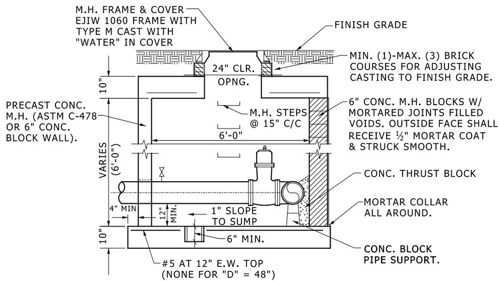
NOTE: STRUCTURE TO BE BACKFILLED WITH CLASS II GRANULAR
