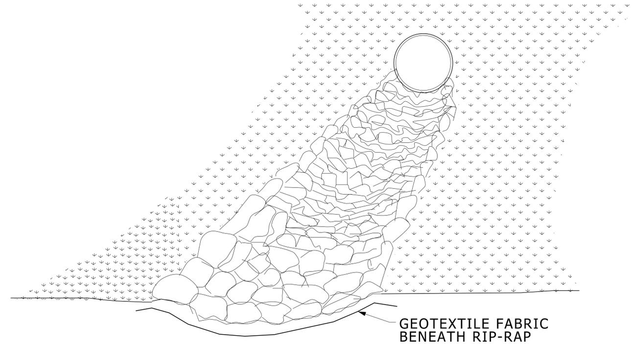
1. MATERIAL USED FOR RIP- RAP SHALL BE SOUND, TOUGH, DURABLE AND FREE FROM STRUCTURAL DEFECTS, AND MAY CONSIST OF STONE, ROCK, OR COBBLESTONE WITH AT LEAST ONE DIMENSION OF 8 INCHES AND A VOLUME OF NOT LESS THAN  $\frac{1}{3}$  OF A CUBIC FOOT. SMALLER PIECES MAY BE USED FOR FILLING VOIDS AFTER LARGER PIECES HAVE BEEN SET.
