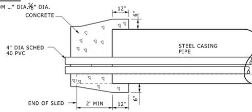
**METHOD FOR SEALING CASING ENDS**
