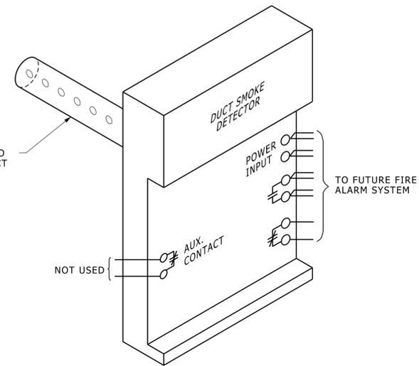
**DUCT SMOKE DETECTOR INSTALLATION DETAIL**
