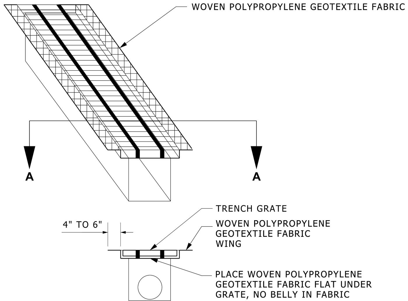
**SECTION A-A TRENCH DRAIN CROSS-SECTION**
