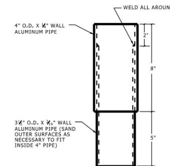
**DETAIL B - LIGHT FIXTURE BASE EXTENSION SINGLE GLOBE FIXTURE**
