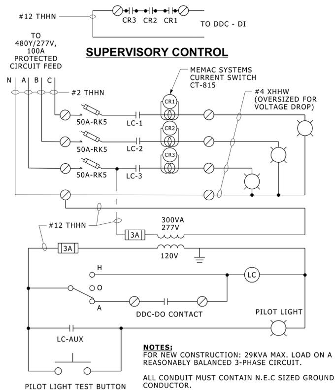
**CONTROL WIRING FOR CONTACTOR**
