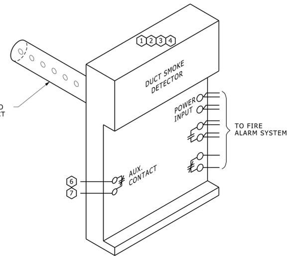
**DUCT SMOKE DETECTOR INSTALLATION DETAIL**
