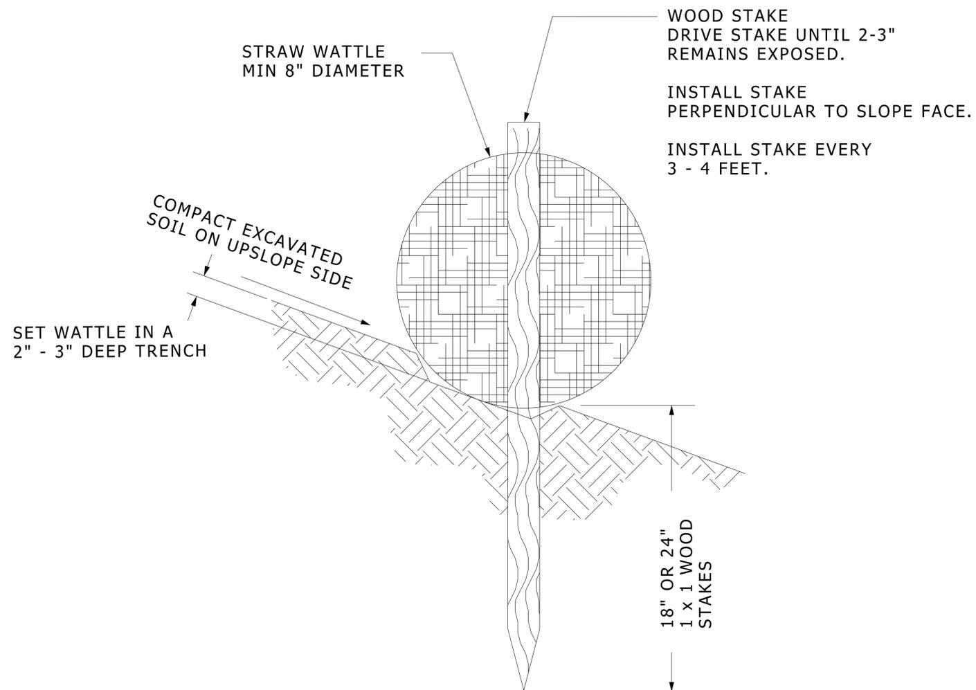
1. BEGIN AT THE LOCATION WHERE THE WATTLE IS TO BE INSTALLED BY EXCAVATING A 2-3" DEEP X 9" WIDE TRENCH ALONG THE CONTOUR OF THE SLOPE. EXCAVATED SOIL SHOULD BE PLACED UP-SLOPE FROM THE ANCHOR TRENCH AND COMPACTED.
