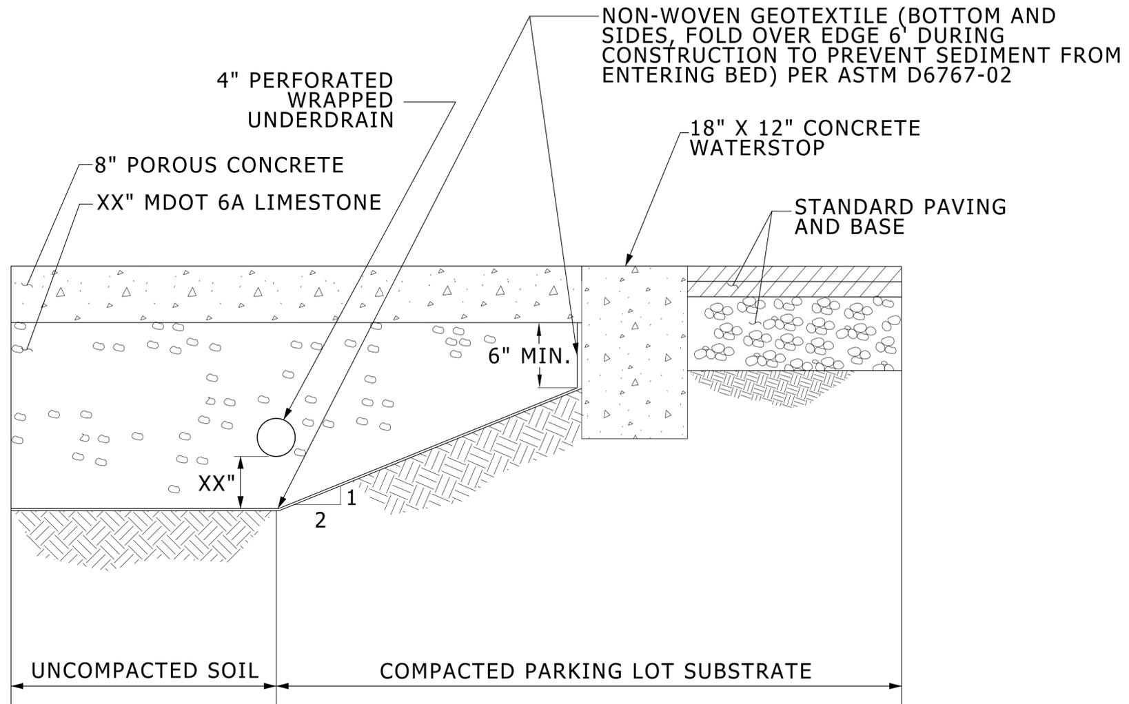
NOTE: INSTALL WATERSTOP BETWEEN PERVIOUS PAVEMENT AND STANDARD PAVEMENT AREAS
