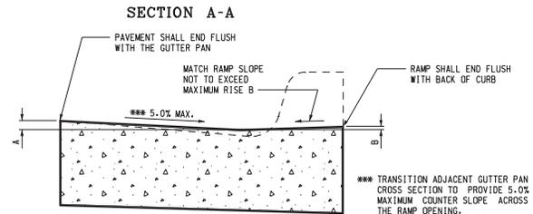
**SECTION THROUGH CURB RAMP OPENING**
