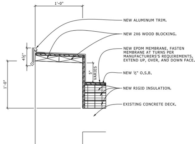
• Optional Roof Edge Detail **ROOF EDGE DETAIL**
