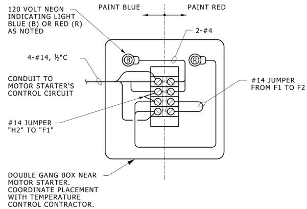
**DUCT SMOKE DETECTOR TO TEMPERATURE CONTROL INTERFACE BOX DETAIL**
