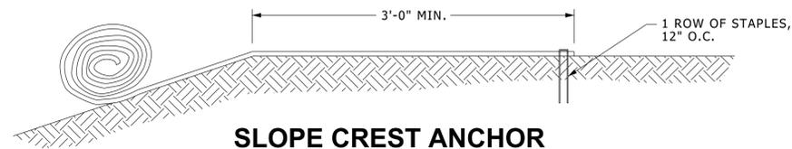
**SLOPE CREST ANCHOR METHOD "A" (NO TRENCH)**
