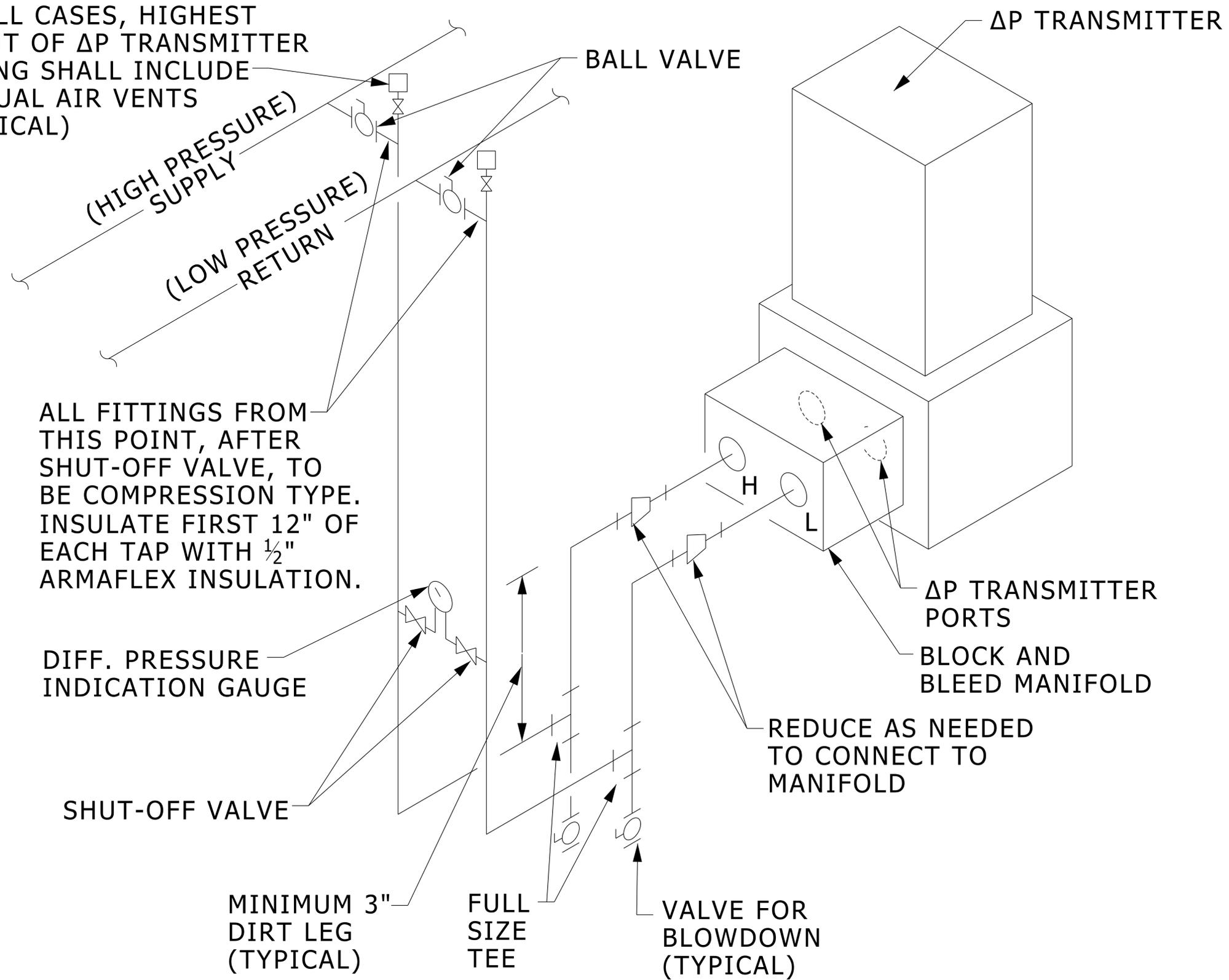
ALL FITTINGS FROM THIS POINT, AFTER SHUT-OFF VALVE, TO BE COMPRESSION TYPE. INSULATE FIRST 12" OF EACH TAP WITH 1/2" ARMAFLEX INSULATION.
