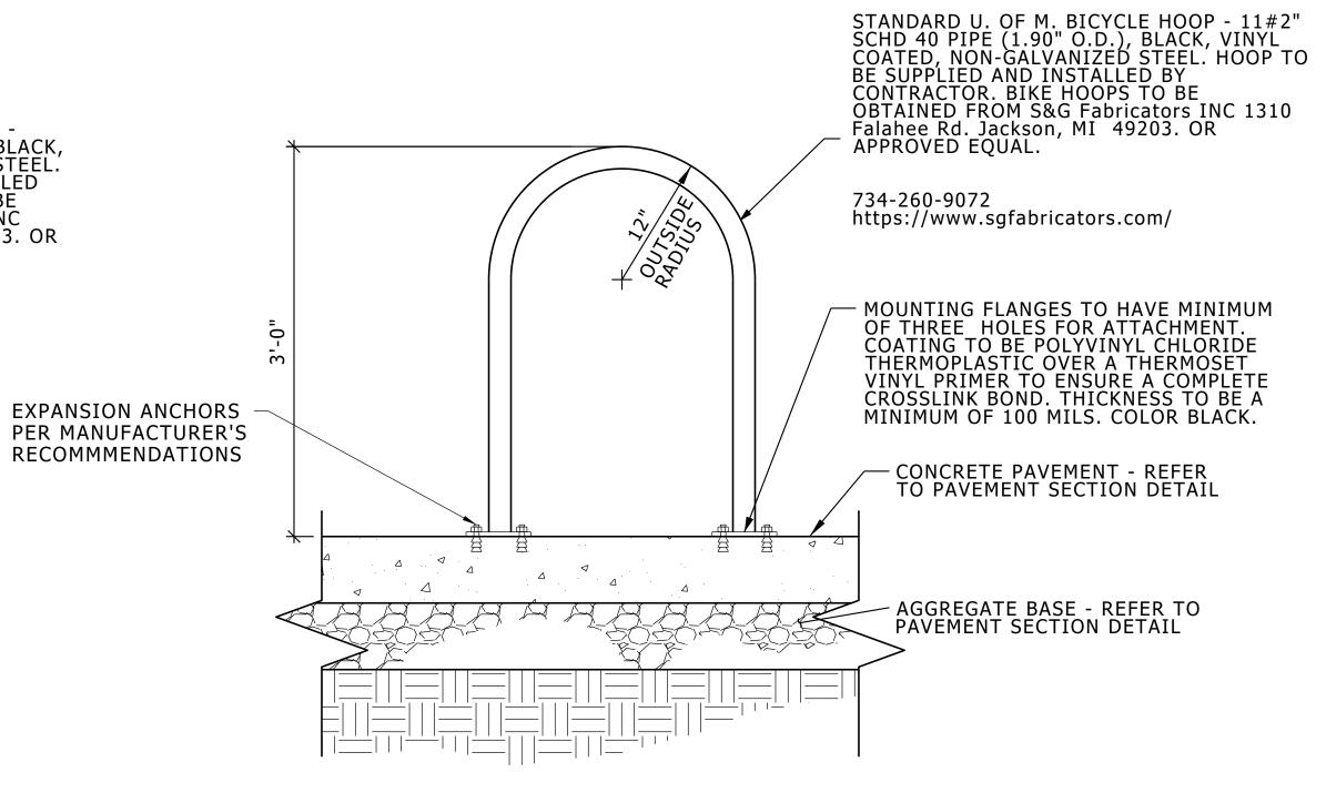
NOTE: STANDARD U. OF M. BICYCLE HOOP. BIKE HOOPS OBTAINED FROM S&G FABRICATORS IN DEXTER, MI OR APPROVED EQUAL
