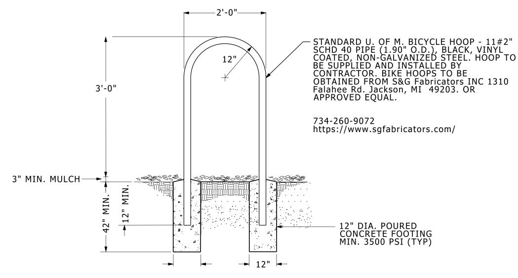
NOTE: STANDARD U. OF M. BICYCLE HOOP. BIKE HOOPS OBTAINED FROM S&G FABRICATORS IN DEXTER, MI OR APPROVED EQUAL
