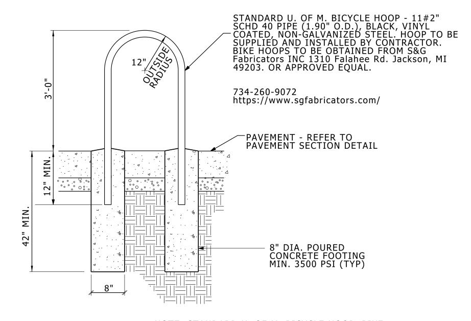
NOTE: STANDARD U. OF M. BICYCLE HOOP. BIKE HOOPS OBTAINED FROM S&G FABRICATORS IN DEXTER, MI OR APPROVED EQUAL
