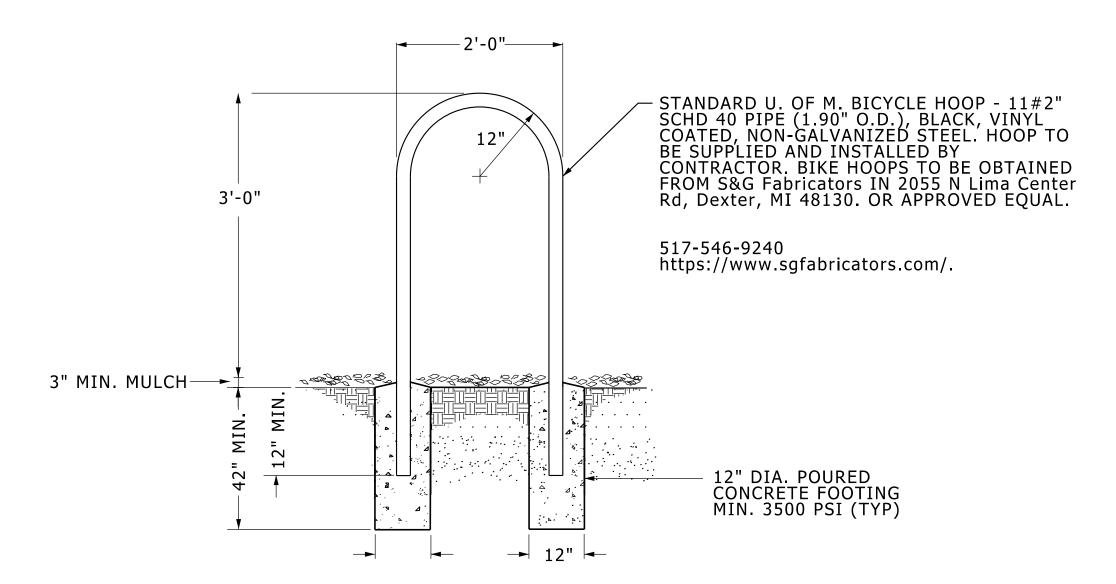
NOTE: STANDARD U. OF M. BICYCLE HOOP. BIKE HOOPS OBTAINED FROM S&G FABRICATORS IN DEXTER, MI OR APPROVED EQUAL
