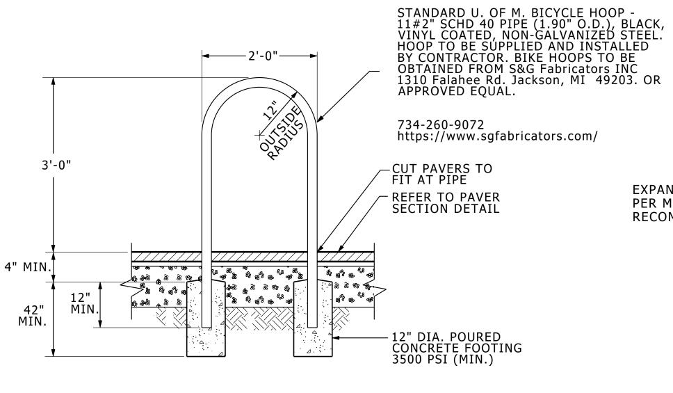
NOTE: STANDARD U. OF M. BICYCLE HOOP. BIKE HOOPS OBTAINED FROM S&G FABRICATORS IN DEXTER, MI OR APPROVED EQUAL
