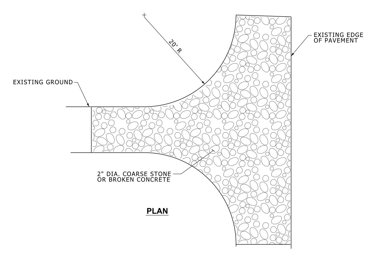
NOTE: CONTRACTOR TO INSTALL & MAINTAIN ANTI-TRACKING PAD. WHEN AGGREGATE BECOMES SATURATED WITH FINES, CONTRACTOR TO SCARIFY AND RELAY AGGREGATE. ANTI-TRACKING PAD DOES NOT RELIEVE CONTRACTOR FROM SWEEPING AND CLEANING ADJACENT WALKS AND ROADS. CRUSHED/BROKEN CONCRETE IS TO BE REMOVED AND LEGALLY DISPOSED OF OFF U-M PROPERTY UPON PROJECT COMPLETION.
