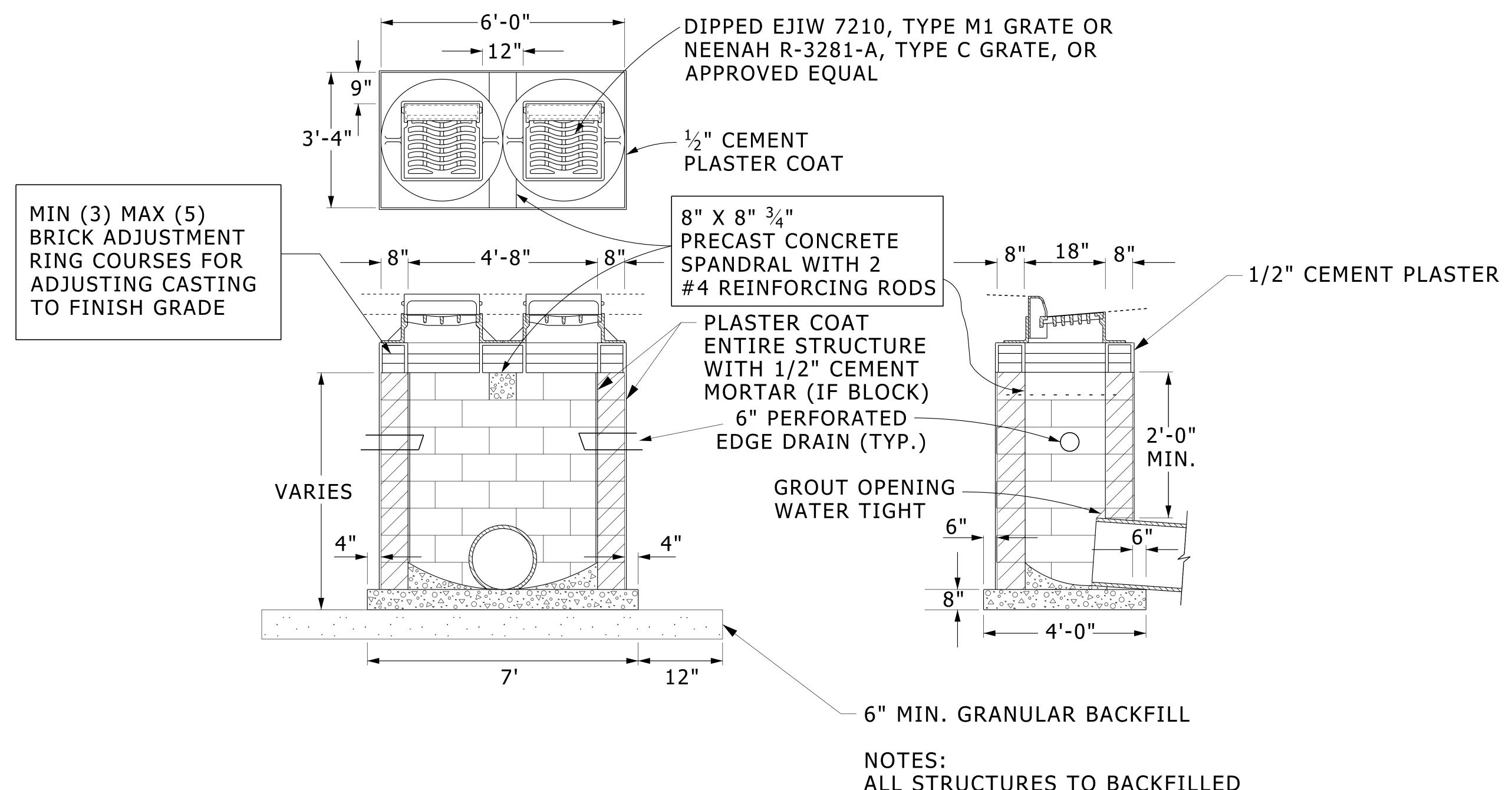
ALL STRUCTURES TO BACKFILLED WITH CLASS II FILL OR 21AA LIMESTONE COMPACTED TO 98% MAXIMUM DENSITY.
