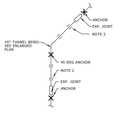
45-DEG TUNNEL BEND ANCHOR PIPING CONFIGURATION
