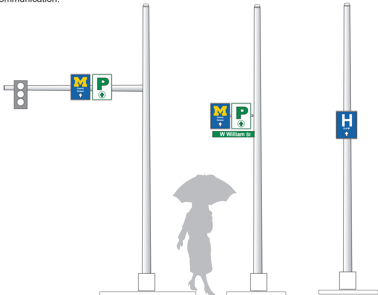
Typical mounting configurations
